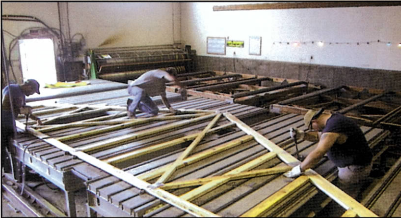
Factory Built Trusses – standard in all building, make a stronger and more precise building.
